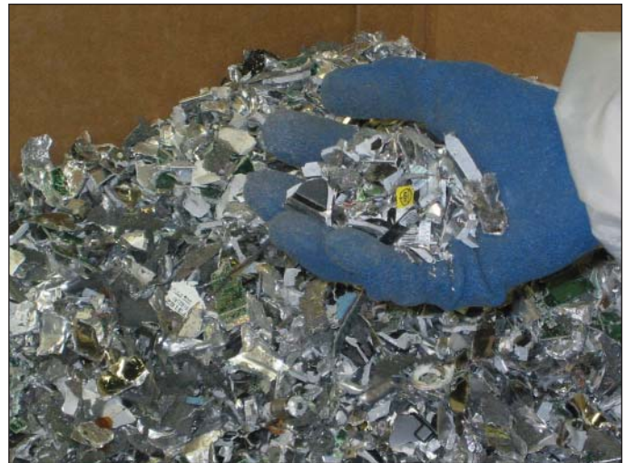
Figure 1: Combining in-house software erasure of hard drives with off-site physical shredding at a secure facility that certifies destruction ensures media is properly destroyed.
